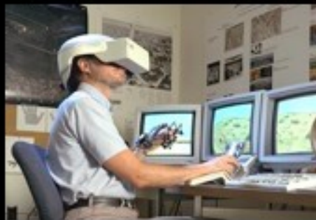
Person with a head-mounted display (HMD), wired glove and joystick. Image
