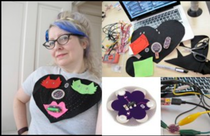
And for looking at social interaction - "Yr In Mah Face": temperature /mood sensing t-shirt - uses Celsius temperature data from a sensor, averages it, then visualises the results via LEDs
